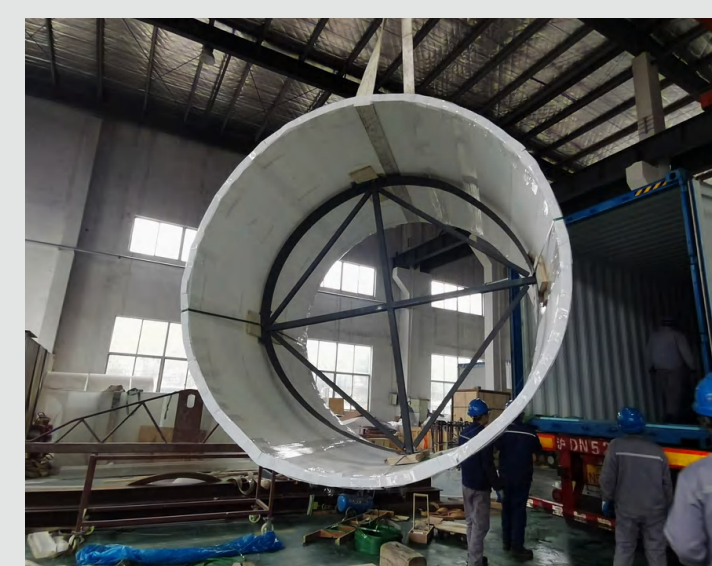
Dubai Swimming Pool Project: 120/160mm thick pool bottom and side panels, 5 pieces in total
